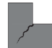
No Claim will be entertained for cracking/peeling of corner or L-Shape
